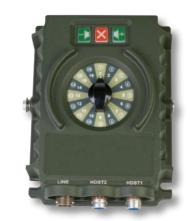
All units feature the same easy-to-use three-button warning and volume control system. The center red button lights to indicate a pending warning status: the two green buttons—used for adjusting headset volume—send an alarm when pressed simultaneously, overriding voice transmissions from all but the alerting unit.
